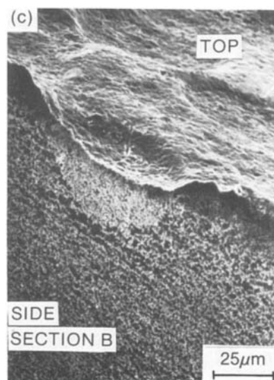
Figure 5 Wetting test with Al-Si eutectic alloy at 590° C: (a) top section of the SiC/Al plate after the wetting test, (b) cross-section of segment A-A revealing the penetration of the Al-Si into the SiC/Al, and (c) high concentration of SiC whiskers collected at the eutectic alloy/composite interface.
